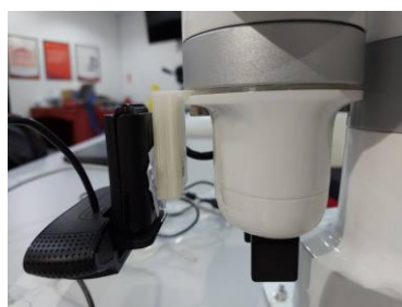
Figure 5. Installation of camera mounting plate on end-effector.
